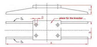
The welding brackets are available in grounded steel or in <u>pickling stainless steel</u>. For stainless steel types please order with ending ...-RF
